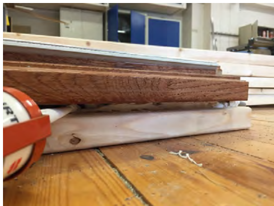
Figure 7. Application of silicon compound.
