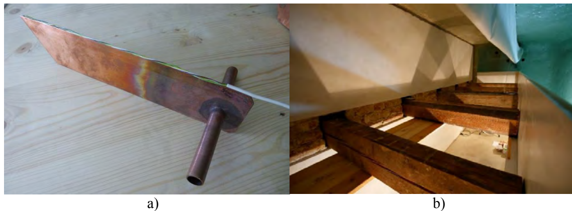
Figure 3. a) Prototype of heat conducting sheet, b) overhead beams without floor assembly
