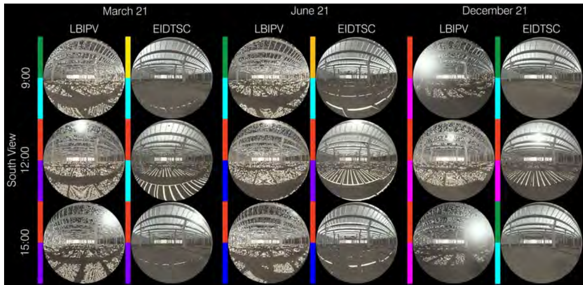
Figure 4. Daylight Glare Probability and Daylight Glare Index from a South facing viewpoint for the LBIPV and EIDTSC canopies at the solstices and spring equinox.
