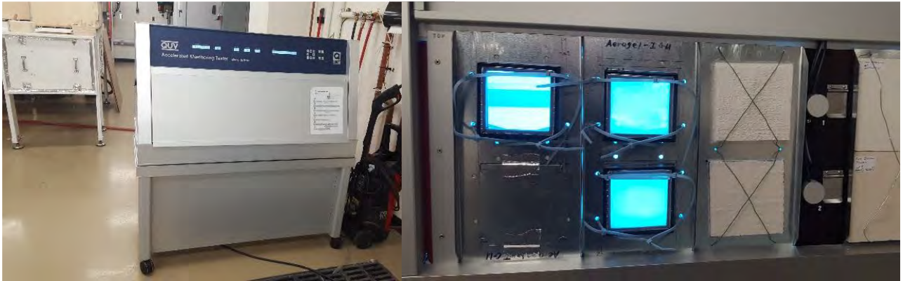
Figure 3. QUV accelerated weathering tester for studying the effects of temperature, moisture, and UV light exposure.
