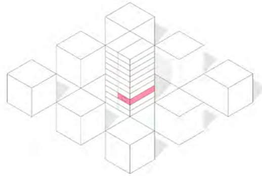
Figure 2: CAD model of the test case. Case one is simulated without contextual obstructions. Case two is simulated as depicted. Red highlights the zone that was modeled in EnergyPlus.
