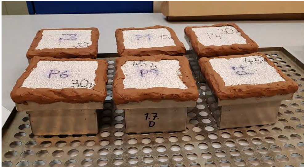
Figure 1. AAC samples for measurement of water vapor resistance diffusion factor.
