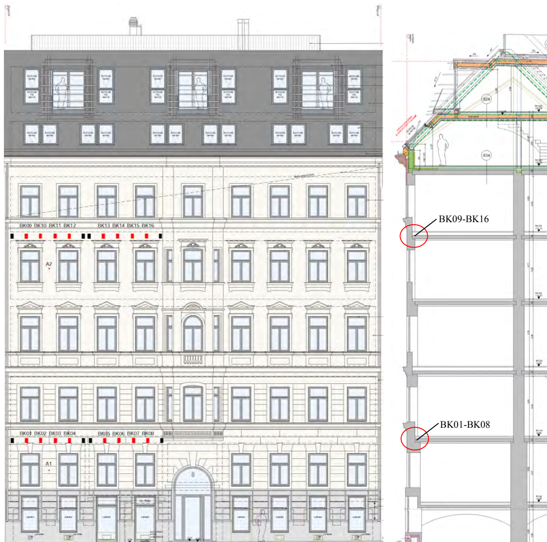
Figure 2. Façade (left) and section (right) of demoobject “Trubelgasse 8” with 16 schematically marked monitored beam heads.
