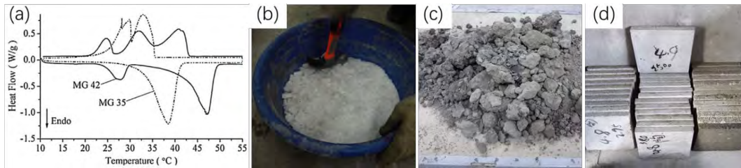
Fig.1 (a) DSC curves of PCMs; picture of (b) Pure PCMs; (c) Composite PCMs; (d) prepared wallboards
