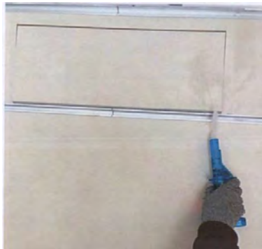
Figure 6: Photograph of smoke test with ventilator in closed position. No air leakage is evident in this condition at any ventilator (left).
