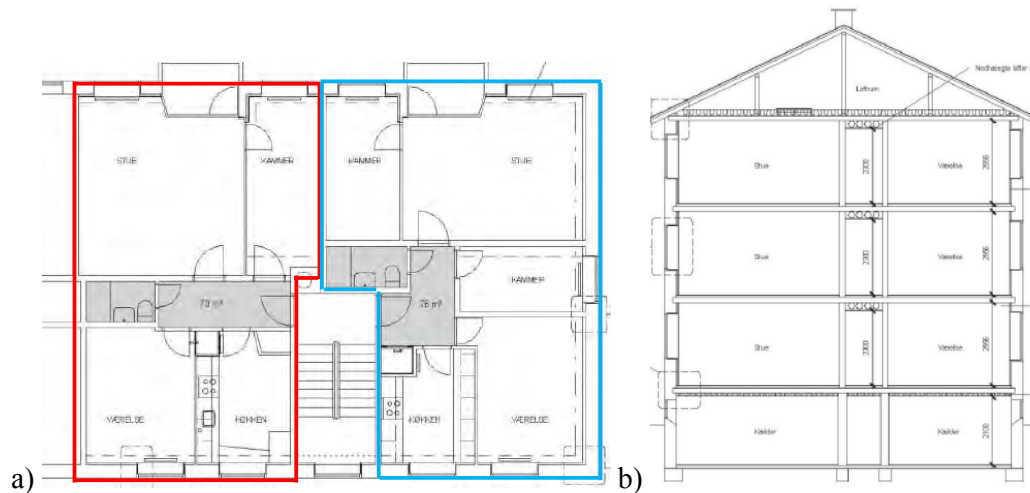
Figure 1. a) Layout of two apartments. Red designation is an internal apartment and blue designation is an apartment with a gable. In the grey area, a suspended ceiling is used to hide ventilation ducts. b) Cross section of the three apartments, basement and attic.
