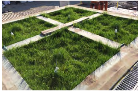
Figure 2. Photo of the four specimens of the investigated vegetated roof in the LIVE.
